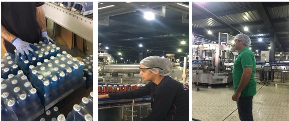
**Figure 7 : Personal Protective Equipment (PPE) used: protective clothing, hairnet, eye protection, and ear protection are worn in the different production areas.**
